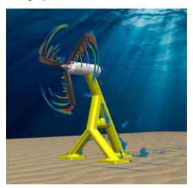
There are many challenges associated with tidal turbines that differentiate them from say wind turbines. For example, the turbulent intensities and length scales associated with their operation are significantly higher than those found around wind turbines. The influence of the turbulent inflow has a dramatic effect on both performance and wake regions, ultimately effecting the model's subsequent accuracy.
